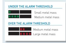
GREEN AND RED METERING SIGNALS PROPORTIONAL TO THE METAL MASS DETECTED
